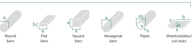
Production method: drawn, extruded, rolled, cast, forged.
